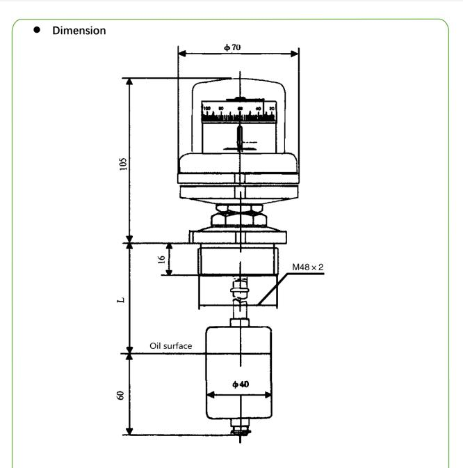
Note: 'L' is the size of the minimum oil level of the transformer and the sealing surface of the mounting screw. Its default value L=120, if there is specified length requirement, please indicate it when ordering.
